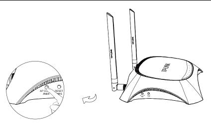
3. Press the AP CLONE/PAIR button on the extender's bottom and the extender's Power LED will blink quickly. In about 20 seconds, both Powerline LEDs will be solid on, indicating that the router and the extender have formed a powerline network. Then both Power LEDs will be solid on, indicating that the AP clone process is completed.
